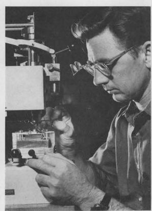
THIS DRILLING machine, operated by James Taylor, can duplicate any pattern of holes from a master plate. Use of such mechanical aids are as close as these machinists come to a "production line."
